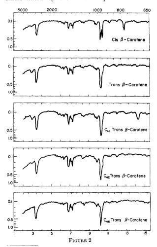
(7) The measurements were made with a Beckman spectrophotometer–Model DU.
